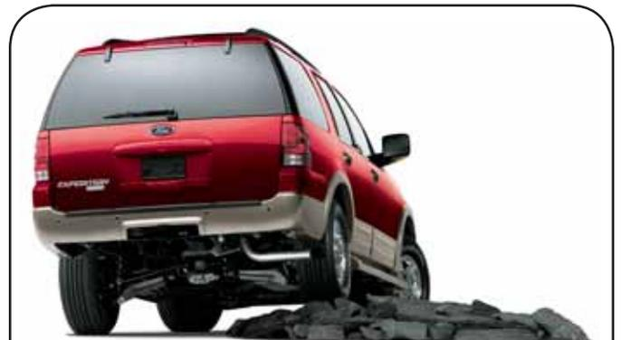
A First-in-Class **Independent Rear Suspension (IRS)** is standard on every Expedition. IRS allows each rear wheel to independently react to changes in terrain, so Expedition is able to maintain its composure when driving over harsh, uneven surfaces.
